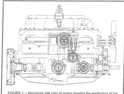
FIGURE 1 - Horizontal side view of engine showing the application of the zoning idea to noise analysis methods.
