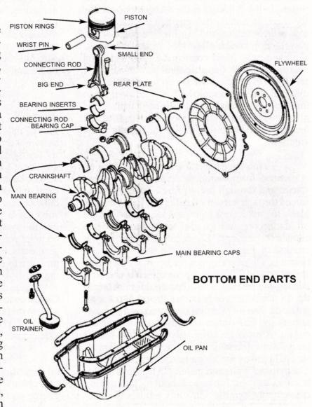
rings. A dry/wet compression test is the easiest way to troubleshoot this noise. Remove the spark plugs and add a tablespoon of engine oil to each cylinder. Crank the engine a few times to distribute the oil past the rings. Install the spark plugs and start the engine. If the noise is reduced, the problem is at the piston ring area.
