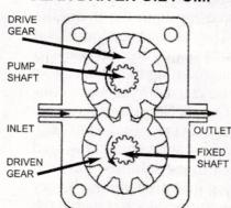
nated and increases oil pump wear. As the pump wears the oil flow is reduced. Generally, in a stock engine, the crankshaft bearings wear out before the pump. There are two types of oil pumps in use: the gear type and the rotor type. Both are driven by a shaft
