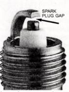
Normal gap growth on a spark plug in a four-stroke cycle engine is 0.00063"-0.000126" per 1000 miles.
