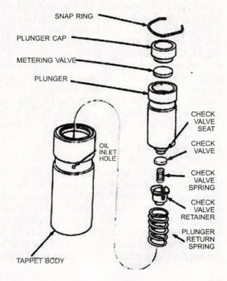
ature is reached. If the noise has quieted down or is gone completely, this is your lucky day. If you start the engine the next day and the noise is still there, the lifters are worn and need replacing. If only one or two lifters are noisy, check for excessive clearances at the rocker arms.
