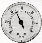
vals, there is a sticking, burnt or leaking valve. A fluttering needle as engine speed increases can be caused by weak or broken valve springs. If a reading drops very low on acceleration, check for an exhaust restriction. Conversely, a very high reading indicates a plugged air cleaner.
