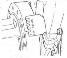
and plug it with a golf tee. Connect the timing light to the number one cylinder. Start the engine, and let it idle. It must idle at a speed that will not engage the centrifugal advance. Aim the timing light beam at the timing marks. Do not get your hand in the fan. Check both centrifugal and vacuum advance. If timing needs adjustment, loosen the distributor clamp bolt, and turn the distributor as required to set the timing marks to specifications. Tighten the distributor clamp, and recheck.
