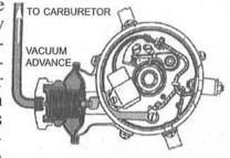
speed and load. The movement of the diaphragm advances the spark the correct amount.
