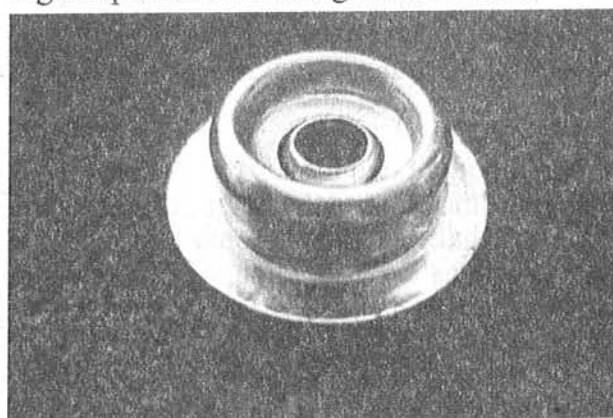
The stud, placed over the eyelet backing plate. The next step is to use the snap installation plier to squeeze the center post and lock the stud, eyelet and leather together. Photo is before the button post was squeezed and locked.
