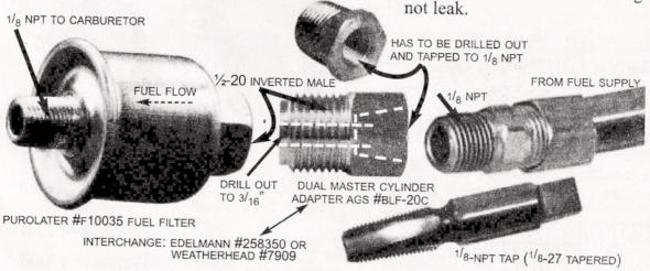
\* For Model A and Model T Fords, vacuum tanks (and other gravity feed fuel systems), be sure that the fuel filter allows fuel to flow freely without the need of pressure to force the fuel through
