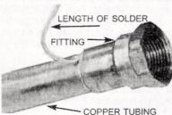
the joint of the two parts. If the metal is hot enough, the solder will be sucked into the joint. Remove the heat and the solder will bond
