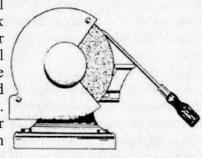
To dress a screwdriver, dress the sides so that they are symmetrical in shape. Then square off the tip of the blade. Check the squareness of the end by resting the blade on a machinist's square. The shank of the screwdriver should be parallel to the handle of the square. Grind the faces of the blade so
