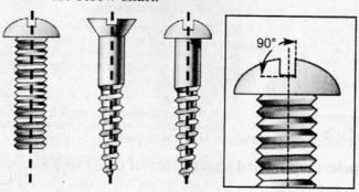
The tip of a screwdriver should fit that slot perfectly. The edge of the blade should be squared and perpendicular to the shaft of the screwdriver. It should not be tapered or chipped. The width of the screwdriver blade should be nearly identical, never wider than, the width of the screw slot. The thickness of the blade should fit snugly into the screw slot.
