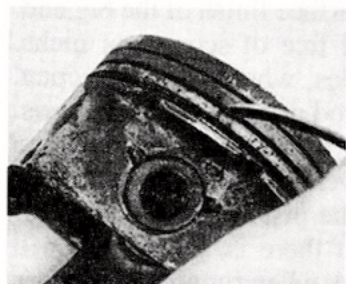
Use a broken ring sharpened to a point to clean carbon from the grooves.
