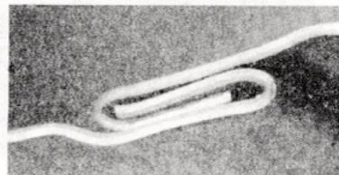
A Pittsburgh lock seam was put onto each end of the sheet metal to lock them together once bent. Not merely a fold in the metal, an offset was made to keep the seam from being too bulky.
