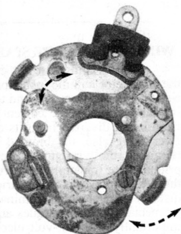
Cars with a vacuum advance have a swivel assembly attached to the top plate.
