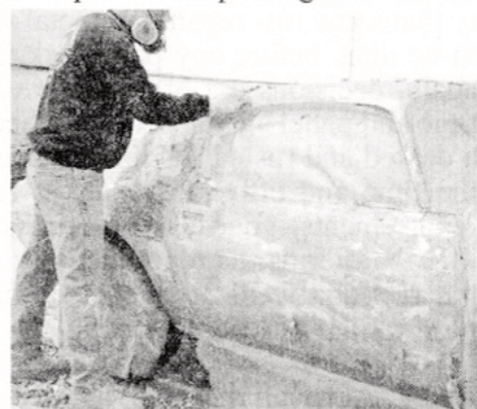
Chemical stripping is a viable option. Note that respirator and goggles are being worn.
